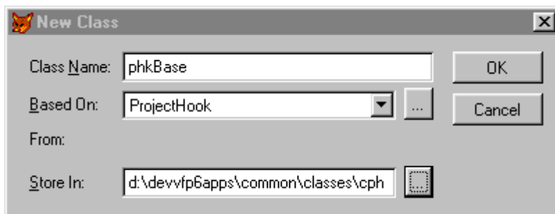
Figure 15.1 The VFP New Class Dialog that demonstrates how to create a new projecthook class
